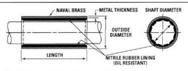
Specially formulated Nitrile rubber compound is used in all standard parts.
